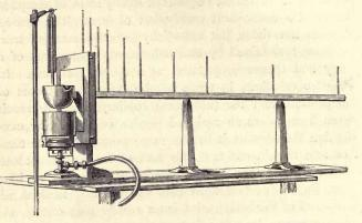
accurate thermometers are inserted, each surrounded by a few drops of mercury. [It is found by calculation based on the results of the experiment itself, that these holes do not, to any perceptible extent, interfere with the transference of heat along the bar.]
